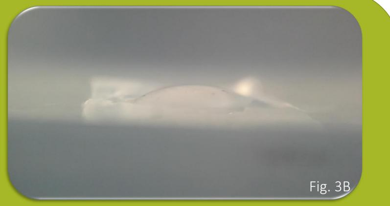
Fig. 3B: Drop of water on a surface of a biomaterial after plasma treatment. The drop changed its shape, flatness is clearly visable.
