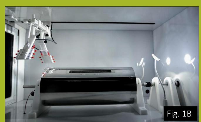
Fig.1A: Electrospinning device; Fig.1B Interior of the electrospining device; Fig. 1C Taylor's cone
